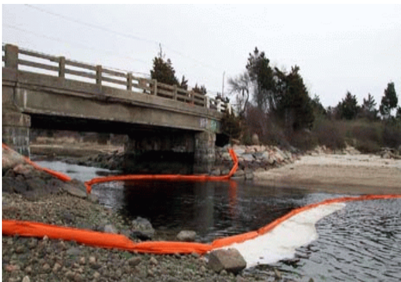
Figure 3.4: Example of a boom deployed in waterbody/channel.
