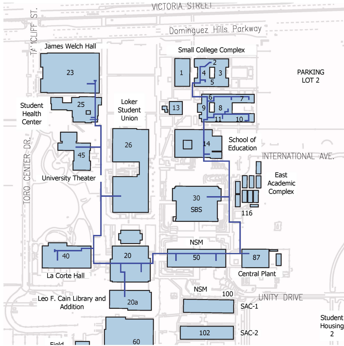
FIGURE 2. EXISTING CHW SYSTEM
