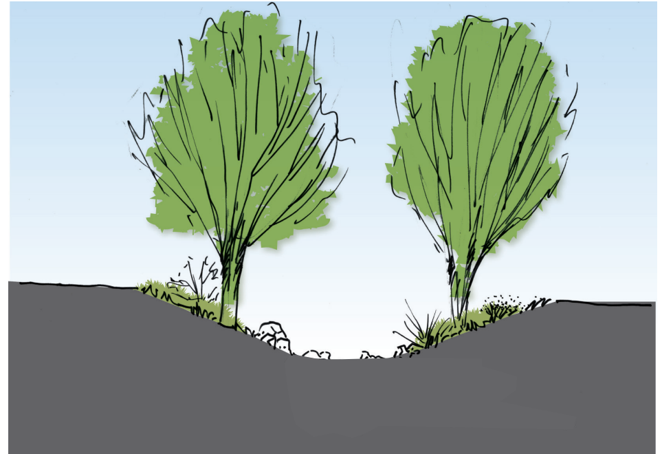
(This diagram demonstrates a typical bioswale)
