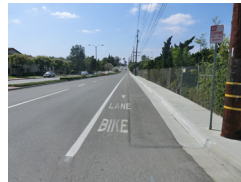
Class II: Bike Lane Provides a striped lane for one-way bike travel on a roadway
