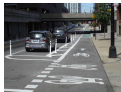
Class IV: Cycletrack Provides a separated right-of-way for the exclusive use of bicyclists adjacent to a roadway
